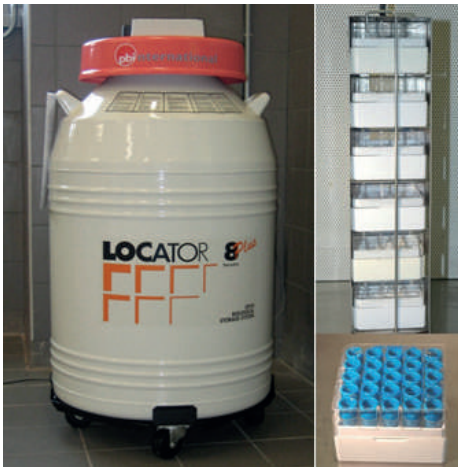
Fig. 27. Locator 8 Plus, dewar for the conservation of samples in liquid nitrogen, for cryobank of Abies nebrodensis germplasm (left); rack and box where cryovials are allocated (right).
