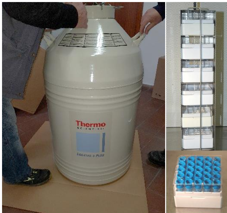
Fig. 7. Left , the Locator 8 Plus, dewar for the conservation of samples in liquid nitrogen, where the cryobank of Abies nebrodensis germplasm will be established; right , rack and box where cryovials are allocated.
