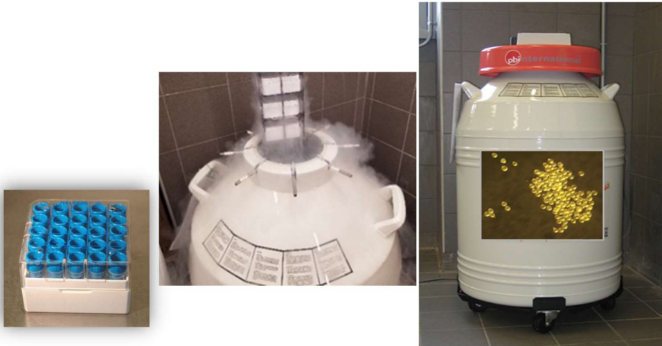
Fig. 5. Pollen in cryovials, immersion and storage in liquid nitrogen (cryopreservation)
