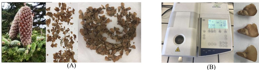
Fig. 1. Extraction and cleaning of seeds (A); Determination of moisture content by Moisture Analyzer (B)
